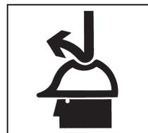
The slug is ejected at the end of the cut. Do not aim cutter or arbor so that ejected slug may hit someone around, or below you.
