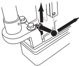
2. With the Clamp Handle Assembly now down, pull the Clamp Handle Assembly clockwise.
