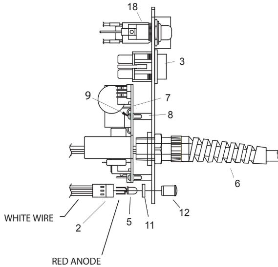
NOTE: WHEN INSERTING L.E.D. DETAIL#5 INTO HARNESS DETAIL#2 MAKE SURE FLAT ON BULB LINES UP WITH WHITE WIRE ON HARNESS.
