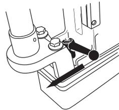
With this being a left handed thread this will loosen this assembly.
