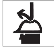
The slug is ejected at the end of the cut. Do not aim cutter or arbor so that ejected slug may hit someone around, or below you.
