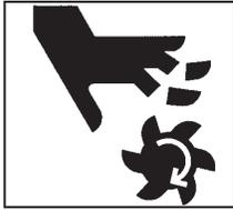
Cutters are sharp. Wear gloves when installing or removing cutter from arbor. Do not grab a rotating cutter.
