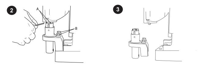
Remove the set screws (A) from the top of the Arbor Body and the Front Support Bracket Bolts (B) from the front of the Magnet. Once these are removed the Arbor Body Assembly can be removed from the Drill Assembly.
