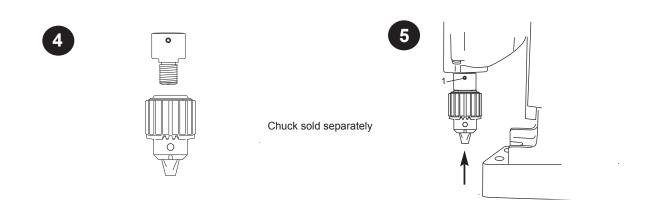
Thread the 3-Jaw Chuck onto the Spindle Adapter until tight. Now slide the complete assembly up onto the Hex Spindle at the bottom of the motor. While pushing up on the Spindle Adapter / Chuck Assembly, turn the set screw in at the top of the Adapter until tight; as shown in Fig.5.
