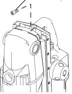
Now that the Chuck and Adapter is installed, part number 40432 Stop Screw needs to be installed on the HMD904 & HMD908 or install the 05357 on the HMD925. This Stop Screw sould be threaded into the top of housing in front of the Motor Assembly as shown in Diagram 6.
